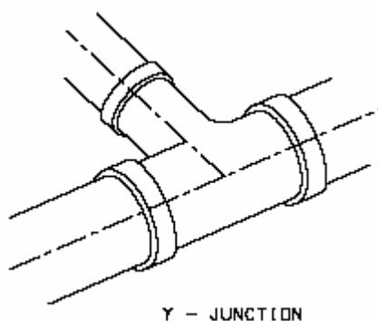
Fig. 3.4 Y-junction in drainage pipes.
