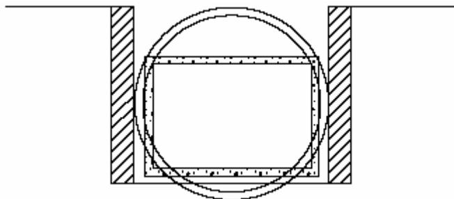
**Fig. 3.1** Small spatial requirement of box culver than pipes.
