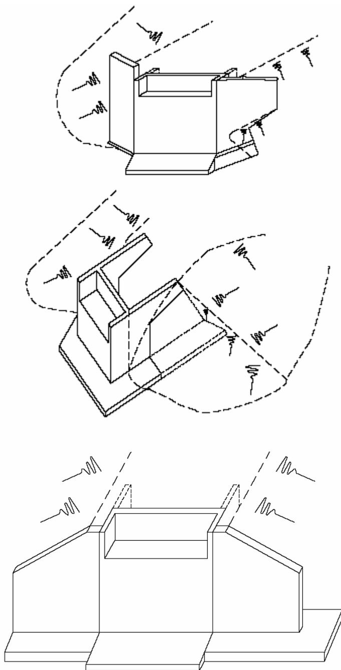
**Fig. 1.4** Different orientation of wing walls.
