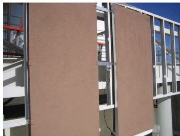
Solar thermal collectors resembling stucco during tests at the University of Nevada, Las Vegas
