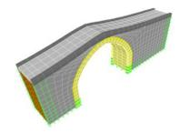
Third mode (Arch vertical movement) f<sub>3</sub>=24.13224Hz
