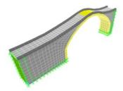
Second mode (Arch vertical movement) f<sub>2</sub>=15.73848Hz
