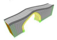
$\label{eq:fifthmode} Fifth mode \mbox{ (Lateral torsional movement)} \ f_5 = 34.22926 Hz$   $Fig. \ 2. \ The \ first \ five \ modes \ of \ the \ Historical \ Pazaryolu \ Bridge \ attained \ from \ the \ analytical \ model$
