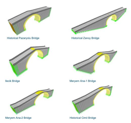
Fig. 1. Pictures belong to three-dimensional analytical model generated in SAP2000  $\,$
