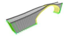
$\label{eq:f5} Fifth mode (Arch torsion movement) \qquad f_5 = 23.98462 Hz$  Fig. 3. The first five modes of the Historical Cimil Bridge attained from the analytical model
