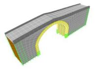
First mode (Lateral movement) f<sub>1</sub>=13.07467Hz
