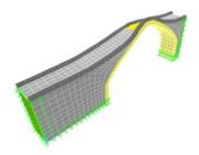
Third mode (Lateral torsional movement)  $f_3$ =16.00709Hz
