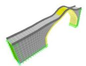
Fourth mode (Longitudinal movement) f<sub>4</sub>=16.26617Hz
