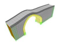
Fourth mode (Longitudinal movement) f<sub>4</sub>=26.61921Hz
