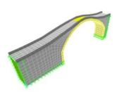
First mode (Lateral movement) f<sub>1</sub>=8.79505Hz
