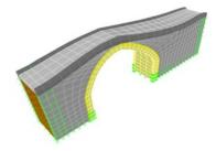
Second mode (Torsional movement) f<sub>2</sub>=23.01439Hz
