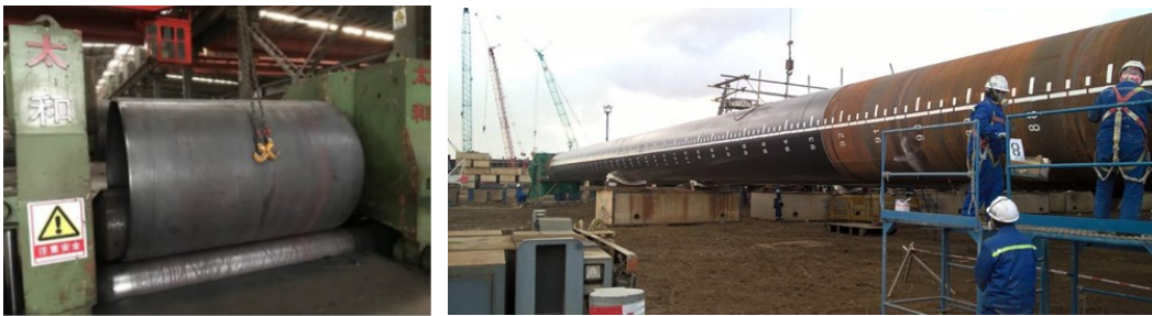
Figure 10. Manufacturing of the piles
