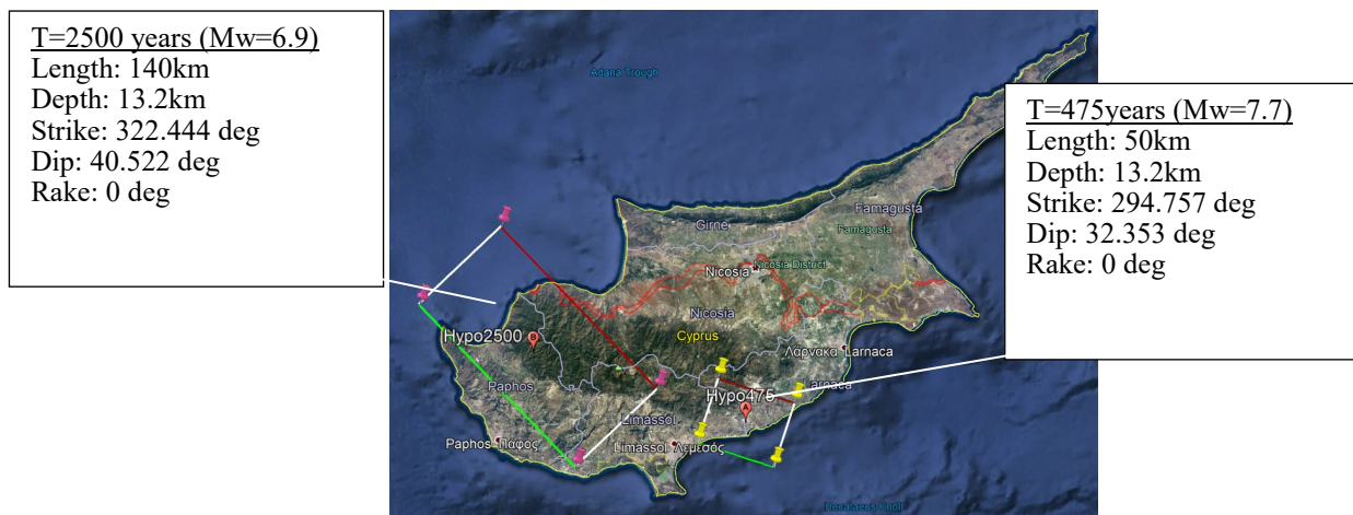
Figure 5. Projected geometry of faults of seismic scenarios on the island of Cyprus (green line depicts top edge of the fault plane, red line bottom edge)
