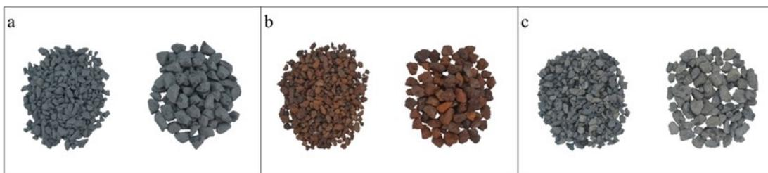
**Figure 1.** The separated aggregates into two groups: (a) CSt, (b) RBA, (c) RCA.
